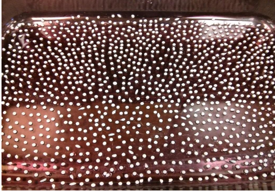
Figure 2.4 CHI-CaP beads separated individually into a dish and air dried overnight at room temperature.
